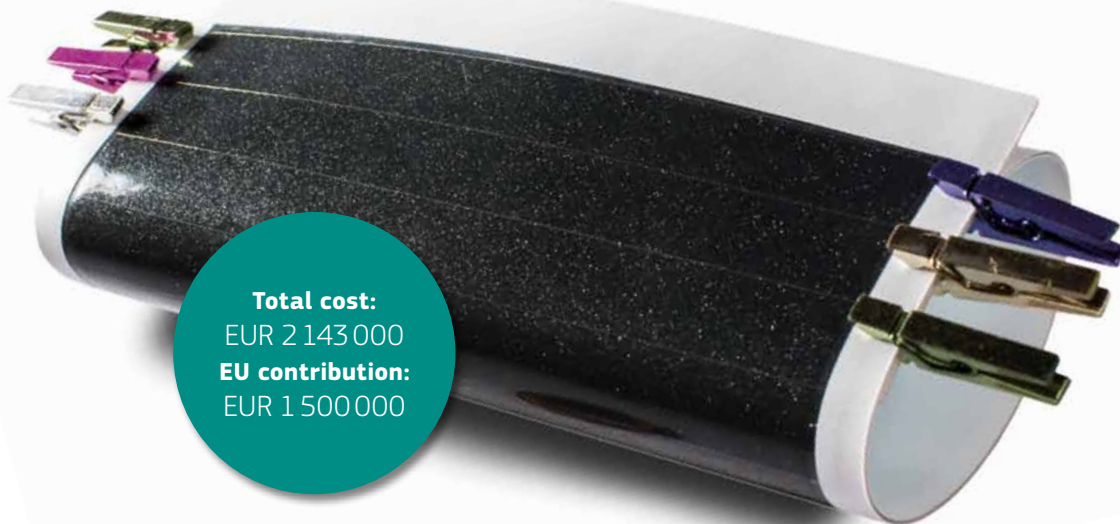
Flexible CZTS photovoltaic film for integration into building elements.
